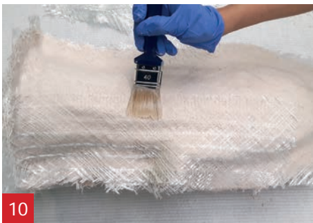
Brush this layer again with A1. Repeat until you have applied 4 layers of A1 Triaxial fibre.
