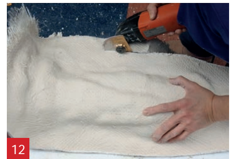
If desired, the A1 support mould can be finished with a multitool.
