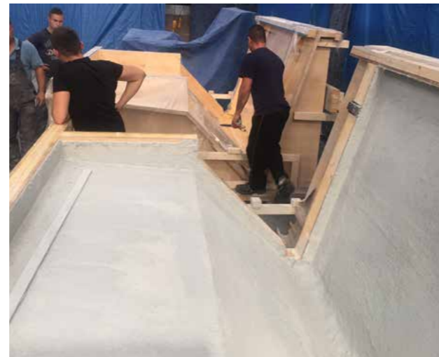
A1 element laminated in the mould
