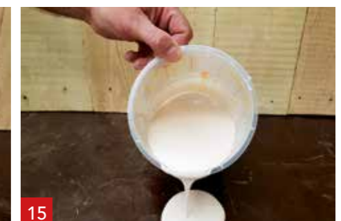
15 A1 is ready for laminating, casting or spraying. Processing time 20 - 25 minutes.
