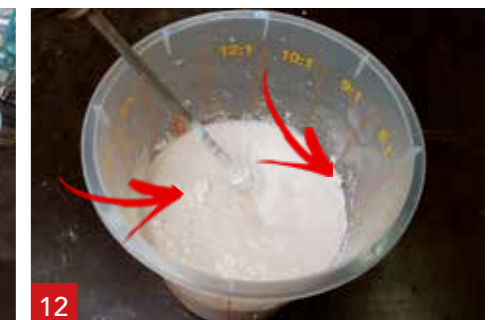
12 Stir the mixer till all lumps have disappeared (± 1 min.) resulting in a smooth material.
