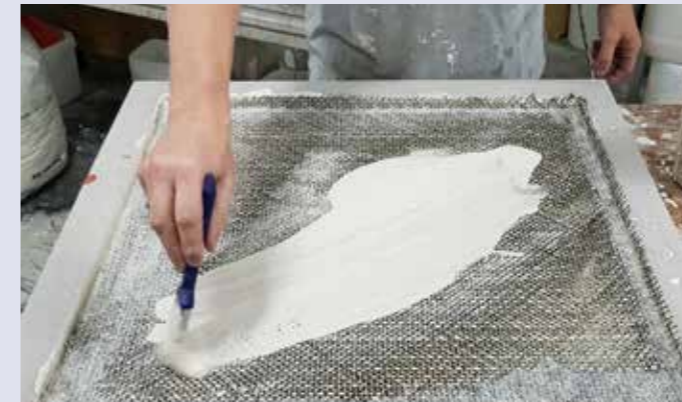
To laminate, you have to work wet in wet. A quick way to apply A1 is with a brush or roller.
