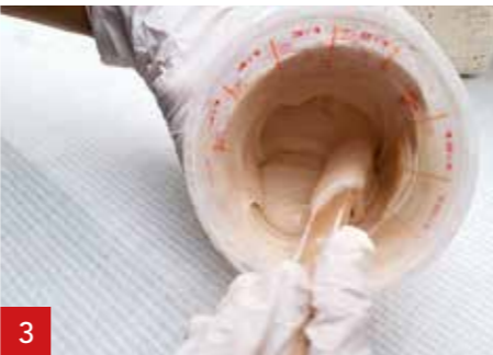
3 Mix the A1 Liquid, Thix A and A1 Powder resulting in a smooth material.
