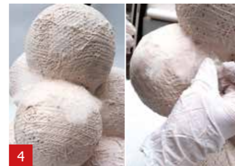
4 Press the small pieces of C-veil into the A1. Overlay the pieces of C-veil.
